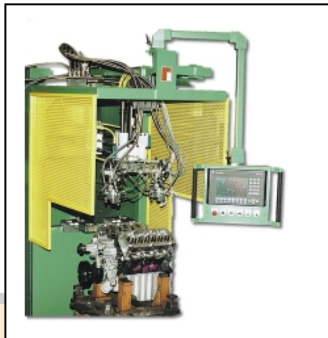
Station 2. Drop Machine with engine block in dispense position
